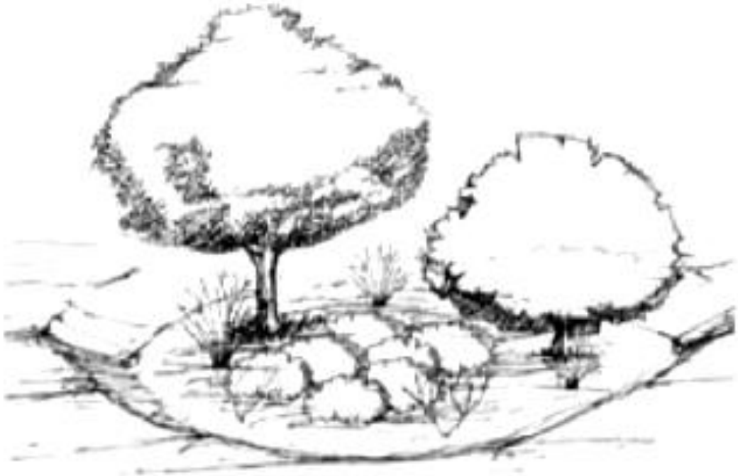
Swales may be used to collect run-off water from a site and to direct it to low-lying areas for passive water retention.
